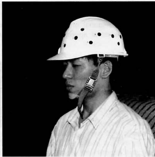
Figure 3 The white helmet was used for precision and accuracy tests. It was attached with 12 black markers of 15mm in diameter.
